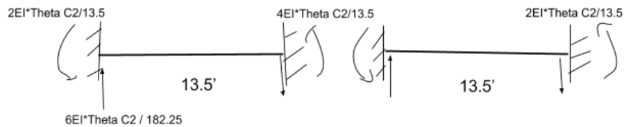
Figure 10: 2 cable slope-deflection \Theta_{C2}
